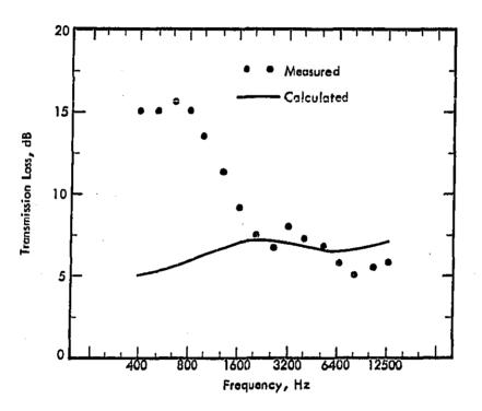
Figure 34. Measured and Calculated Values of Transmission Loss At a "T" Junction.<sup>111</sup>
