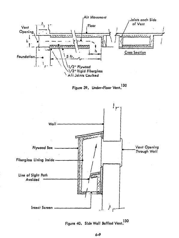
versions of such vents for different applications have been designed and shown to be suitable for protection against high exterior noise levels.<sup>130</sup> They are particularly effective for under-floor areas, and attics. A flow-through system can significantly lower attic temperatures and reduce the energy needed to cool dwellings in the summer months. In some cases, cases, the need for cooling may be eliminated with a combination of natural ventilation and a flow-through attic system.
