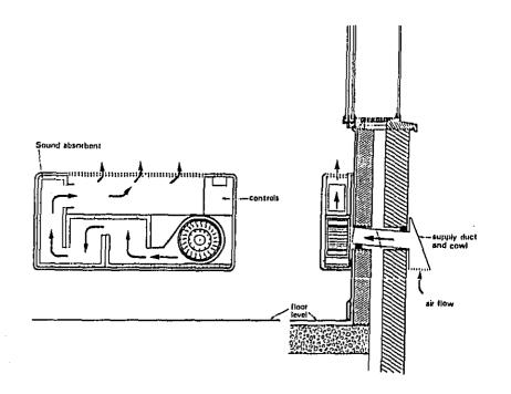
Figure 41. Mechanical Ventilation Unit With Sound-Attenuating Labyrinth.<sup>131</sup>
