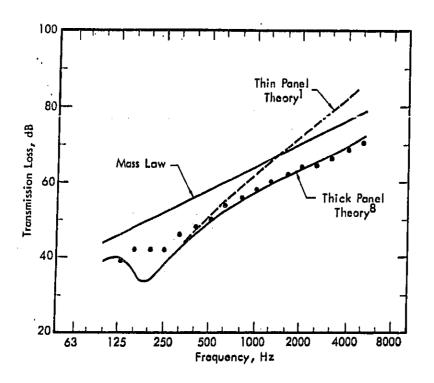
Figure 5. The Measured Values of Transmission Loss for a 15 cm Concrete Panel Compared to Values Predicted by Means of the Thin and Thick Panel Theories.
