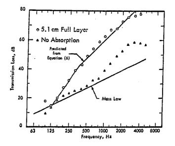
Figure 11. Measured Values of the Transmission Loss of an Isolated Double-Wall Construction With and Without Cavity Absorption. The Construction Consists of 0.64 cm and 0.32 cm Hardboard With a Spacing of 16 cm.<sup>8</sup>
