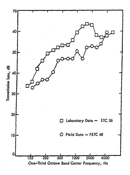
Figure 24. Laboratory and Field Measurements of Transmission Loss For a Wood-Frame Partition With Gypsumboard Mounted on Resilient Channels.<sup>70</sup>
