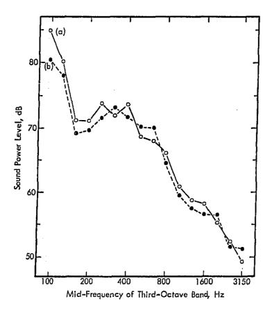
Figure 36. The Total Sound Power Radiated Into The Receiving Room In The First Sound Transmission Experiment; (a) By Independent Method; (b) By Direct Method.<sup>114</sup>
