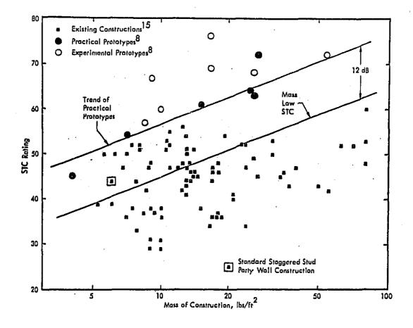
Figure 15. The STC Rating as a Function of the Mass For Existing<sup>15</sup> and Prototype<sup>8</sup> Wall Constructions.
