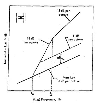
Figure 12. General Form For the Transmission Loss of a Double Panel With Sound Bridges.<sup>8</sup>
