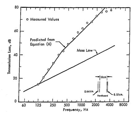
Figure 9. Measured Values of the Transmission Loss of a Double Panel Compared to Values Calculated by the Approximate Method. Fiberglass Batts in the Cavity for Measured Data.<sup>8</sup>
