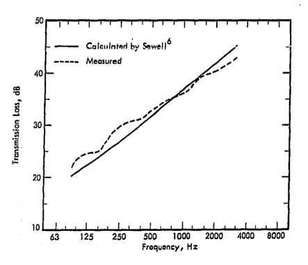
Figure 3. Calculated and Measured Transmission Loss For a Lead Panel.<sup>6</sup>
