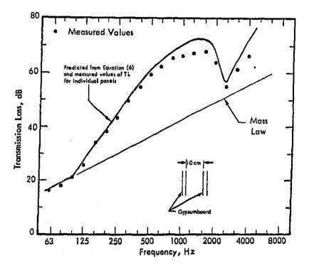
Figure 10. Measured and Calculated Values of the Transmission Loss of 1.59 cm (5/8-inch) Gypsumboard. Fiberglass Batts in the Cavity For Measured Data.<sup>8</sup>
