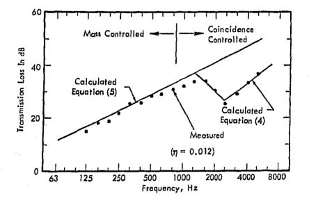
Figure 4. Measured and Calculated Values of the Transmission Loss of 1.59 cm (5/8-inch) Gypsumboard.<sup>8</sup>
