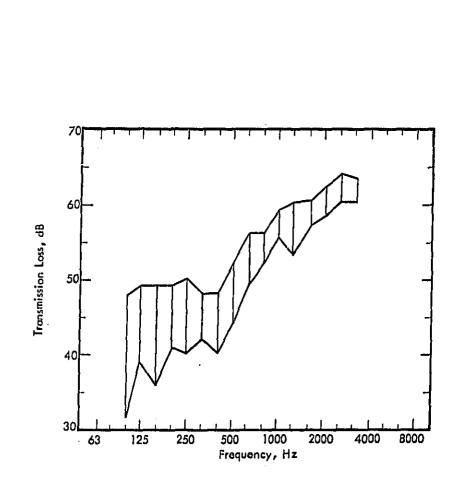
Figure 19. Range of Data Obtained From Measurements on a 23cm Brick Wall By Twelve Organizations in the Same Test Facility.<sup>46</sup>
