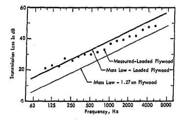
Figure 7. Measured Values of the Transmission Loss of a 1.27 cm Plywood, Panel Mass Loaded to 19.5 kg/m<sup>2</sup> With Asphalt Roofing Paper.
