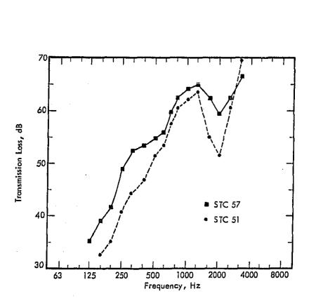
Figure 21. Data Obtained From Measurements on a Wood-Frame Wall With Gypsum Board on Double Row Studs at Two Test Facilities.<sup>4</sup>
